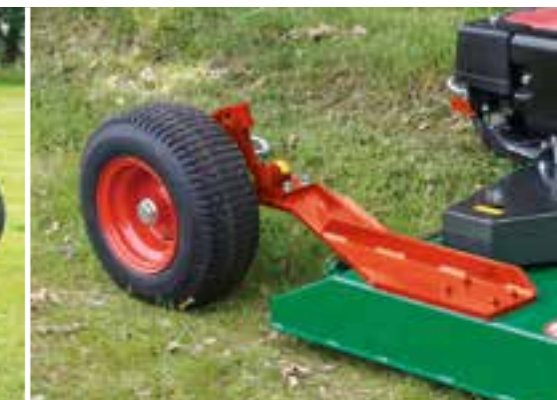
AVAILABLE WITH OPTIONAL REAR WHEEL KIT (AR-120 & AR-150 ONLY), IDEAL FOR MOWING CLOSE TO A FENCE
