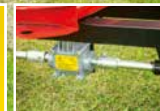
GROUND DRIVEN GEARBOX WITH SPINNER DISENGAGEMENT
